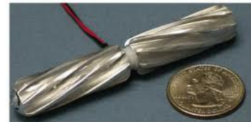
A wireless endolumenal mobile robot like this could one day be used to assist in natural orifice procedures.
